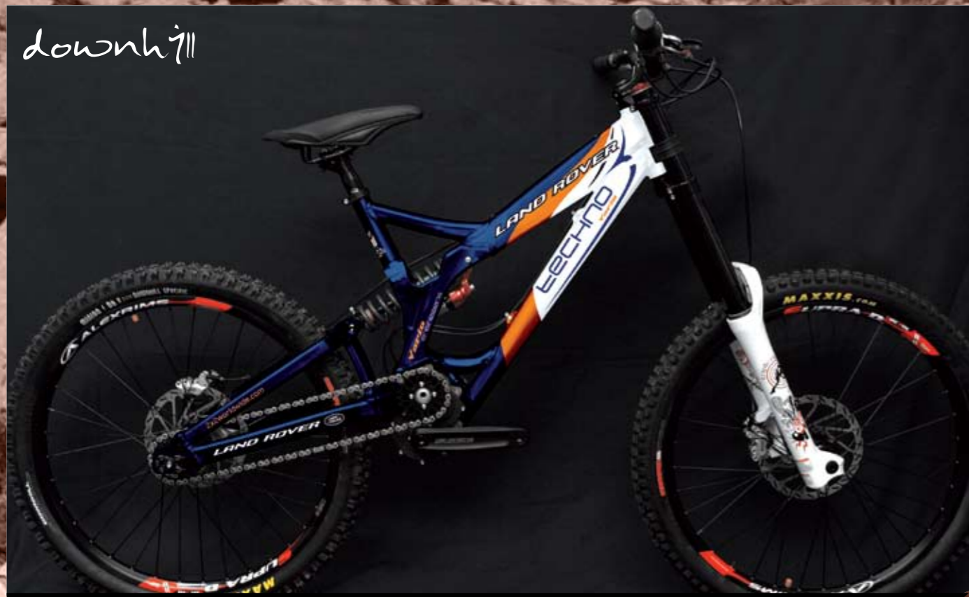
The techno has a professional downhill race frame designed around the new suntour gearbox. Marzocchi, Avid, Truvativ, Maxxis, and Fizik downhill race components are specified, so the bike is finished to the highest of standards for international competition.
